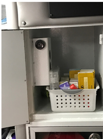
Photo(s): EDGE M-300 Wireless Sensors in ambulance medication cabinet (left) and container (right).
