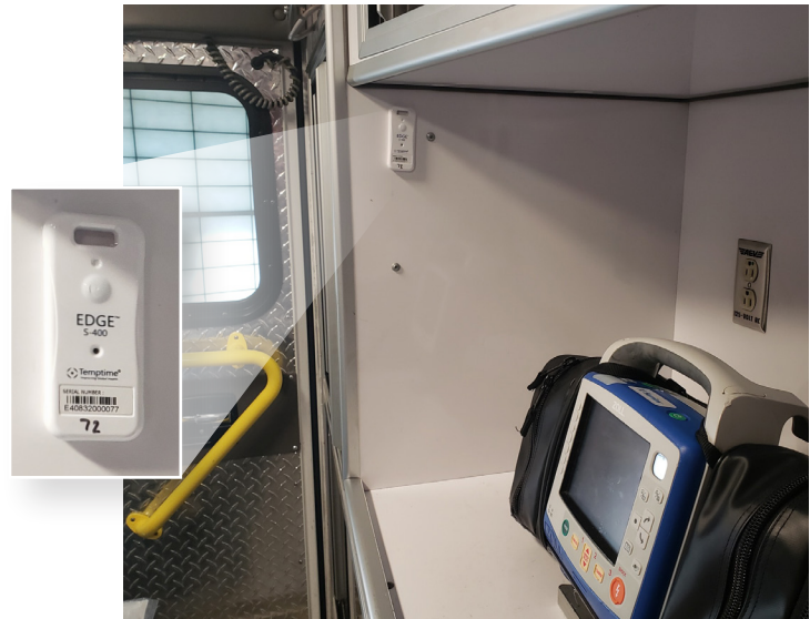
EDGE® S-400 Bluetooth®-enabled sensors are installed in each of MedStar's fleet of 63 ambulances.
